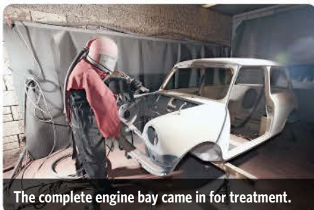
All media must be vacuumed away before primer.
