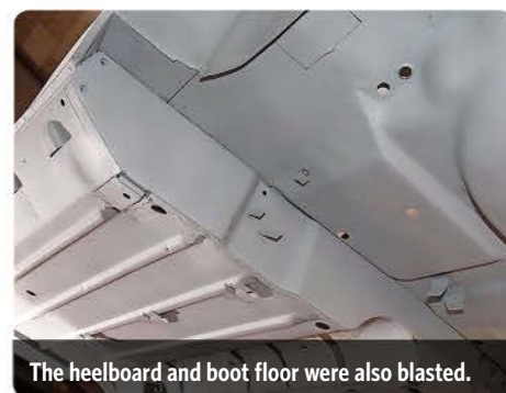
The shell is rotated to get to the underside.
