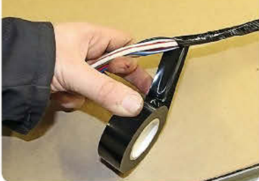
Non-adhesive loom tape pulled taught.
