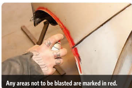
Seams/edges were blasted rather than full panels.
