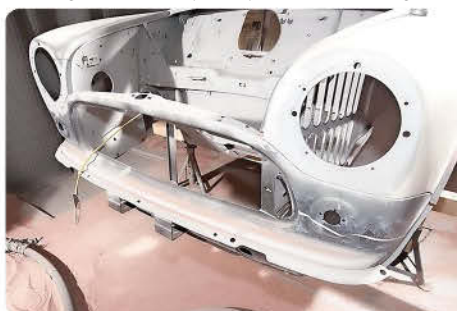
Fully blasted, etch primed and ready for the trip home. It's important to have the shell primed soon after it's blasted to avoid surface rust forming.
