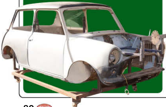
A 360-degree spit allows easy access all round.
